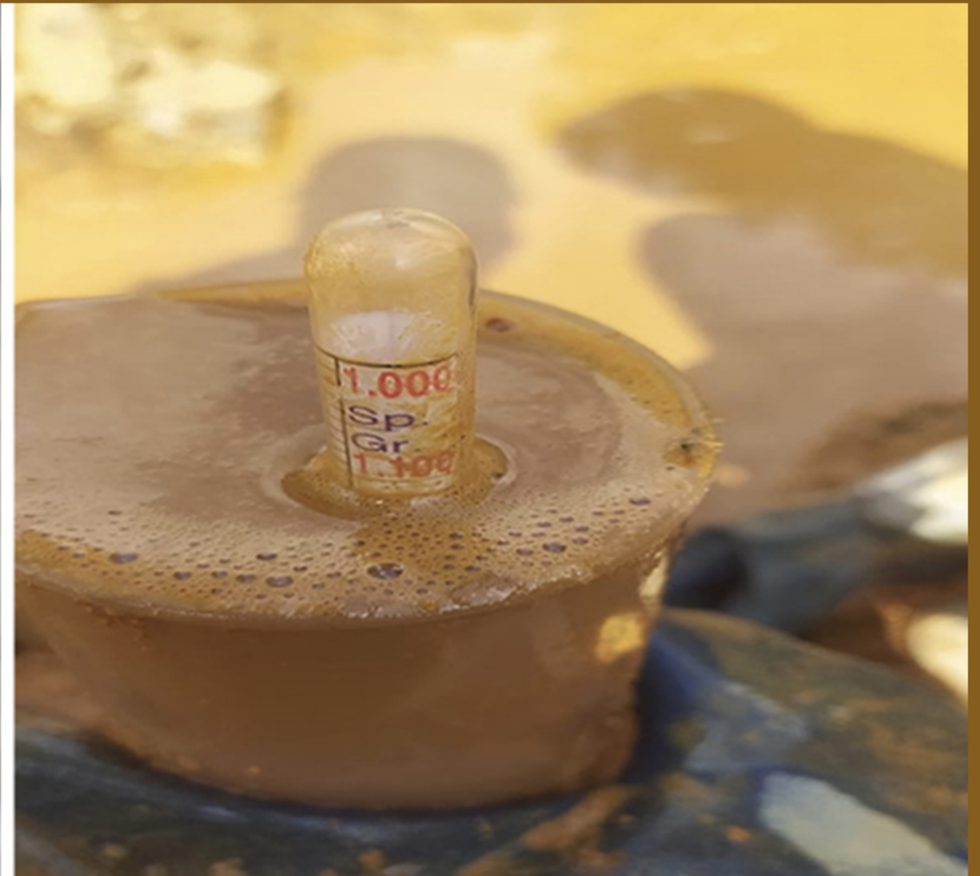
BLOCK B-BENTONITE PIT DENSITY CHECKING
