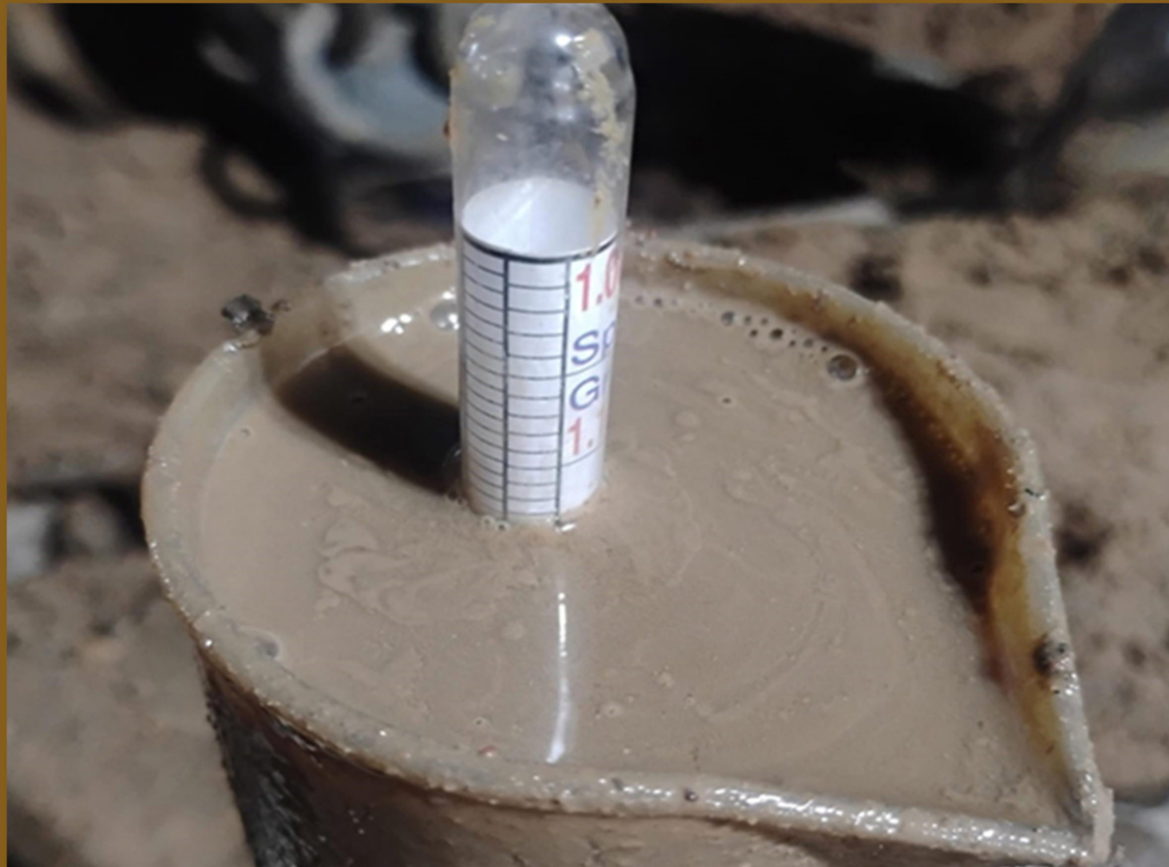
BLOCK B-BENTONITE PIT DENSITY CHECKING
